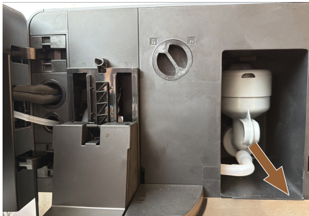
Fig. 88: Pull the mixer forward
