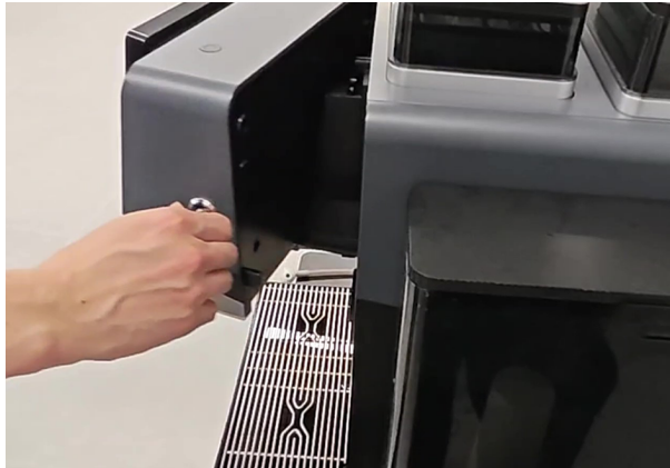
Fig. 128: Open the coffee machine
